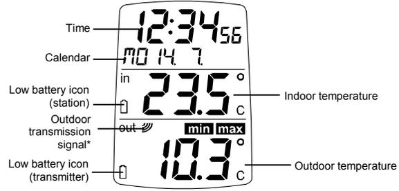
\* When the signal is successfully received by the temperature station, the outdoor transmission icon will be switched on. (If not successful, the icon will not be shown on LCD). The user can then easily see whether the last reception was successful (icon on) or not (icon off). On the other hand, the short blinking of the icon shows that a reception is currently taking place.
